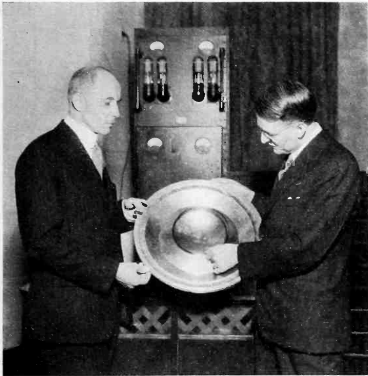
Dr. Frank B. Jewett and Dr. Harvey Fletcher of the Bell Laboratories with one of the low-frequency speaker diaphragms
